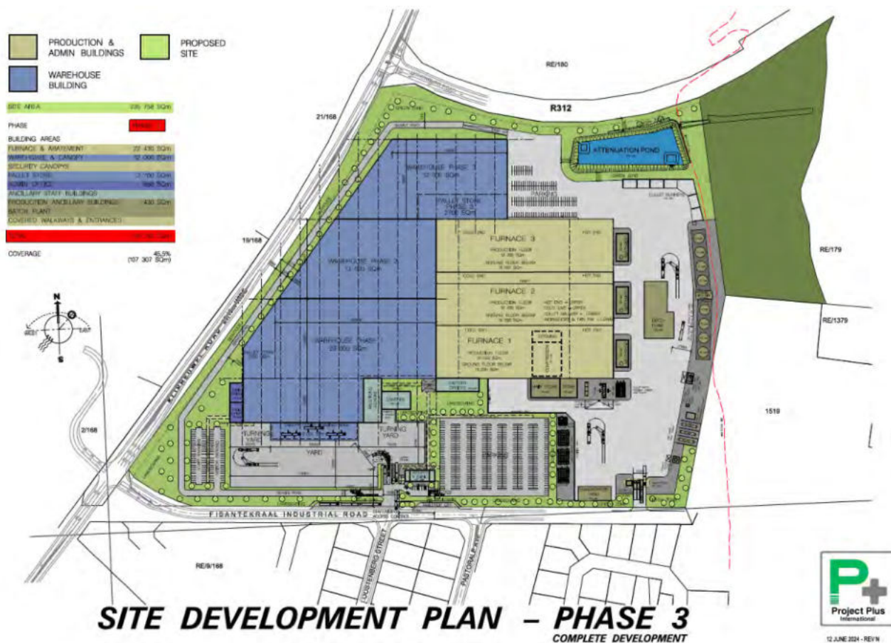
Figure 12: Proposed Cape Speciality Glass (CSG) Development on Remainder Farm 180, Portion 3 of Farm 180 and Portion 13 of Farm 168 (source: Project Plus International)
