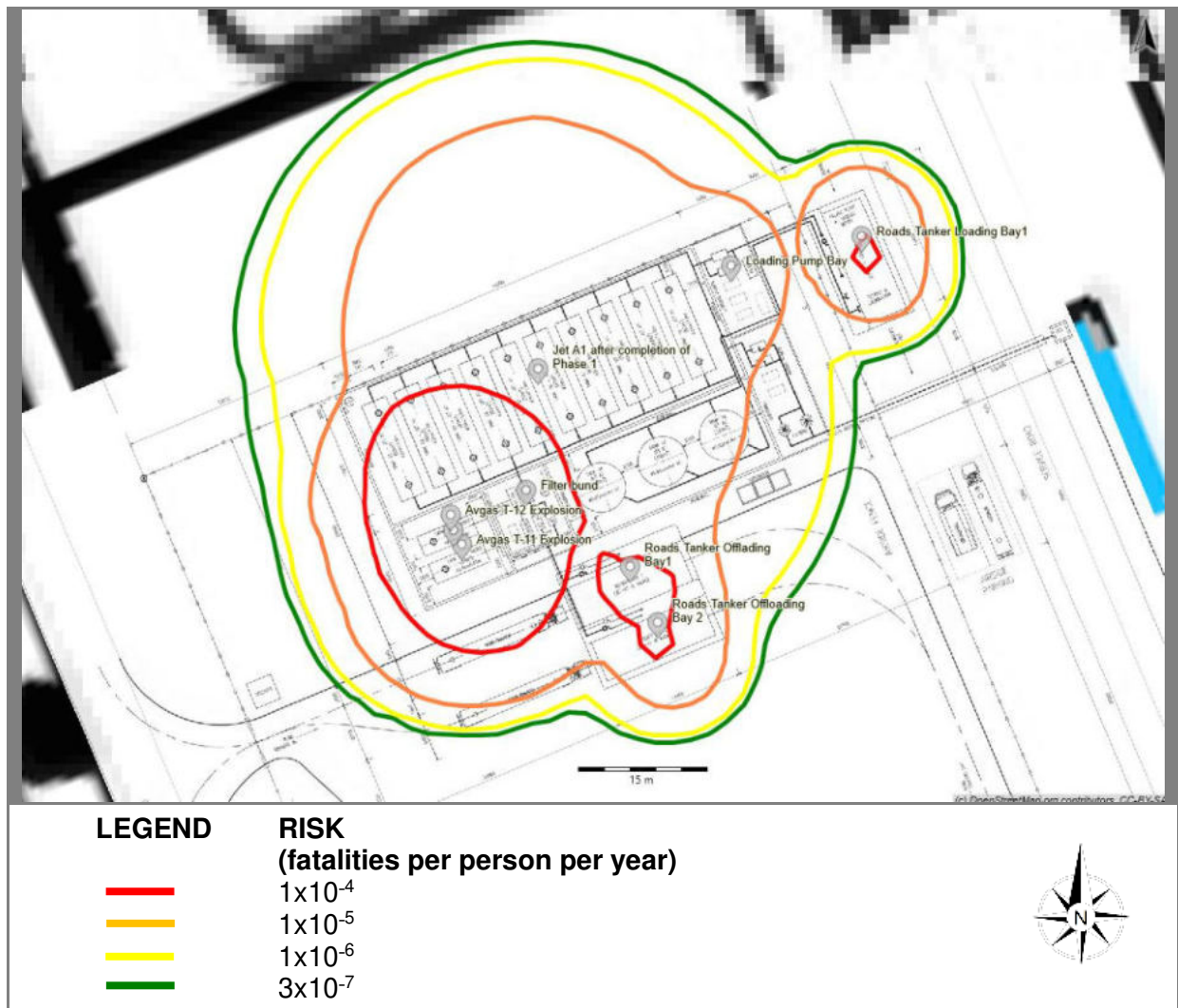
Figure 6-6: Lethal probability isopleths associated with the fuel storage tank farm the end of Phase 2
