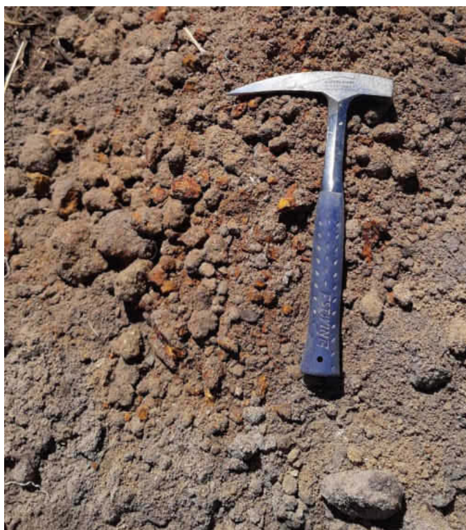
Figure 34: TP11 – Close-up of spoil pile of ferricrete nodules excavated from trial pit.
