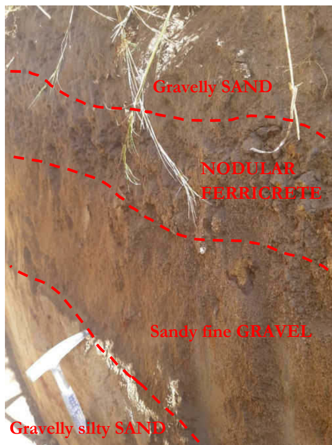
Figure 39: TP15 – Close-up of trial pit sidewall showing various horizons encountered.
