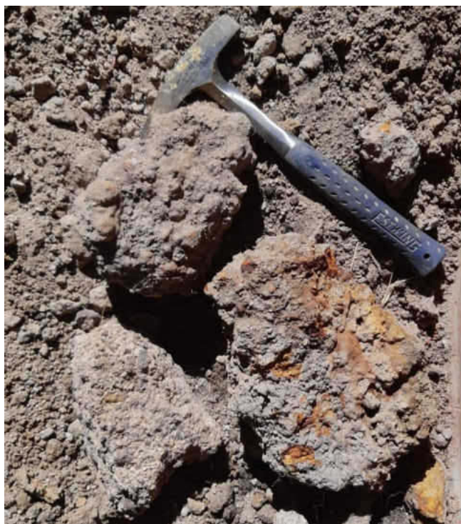
Figure 21: TP04 – Nodular to hardpan ferricrete.
