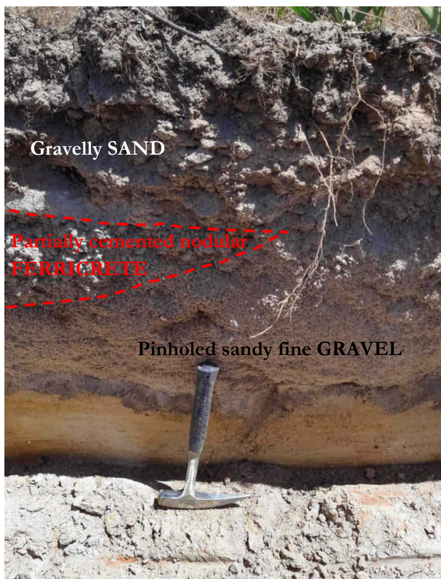
Figure 25: TP05 – Close-up of trial pit sidewall. Note pinch out of nodular ferricrete horizon, and pinholed nature of gravel horizon near base of hammer. Sidewall smear near base indicating high fines content.
