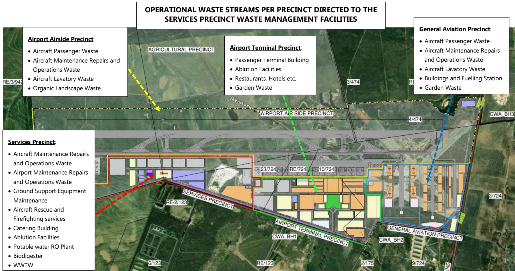
Figure 5: The Phase 2 SDP for the Cape Winelands Airport expansion. All waste streams on the airport will be separated at source from where it will go to the services precinct (red outlined area) for the management of waste on site and where it will be collected for further off-site management.
