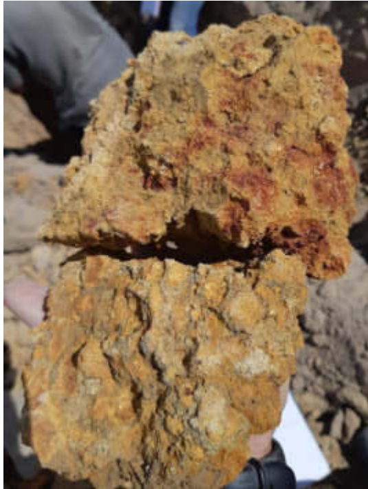
Figure 53: TP32 – Close-up of orange blotched red residual horizon.
