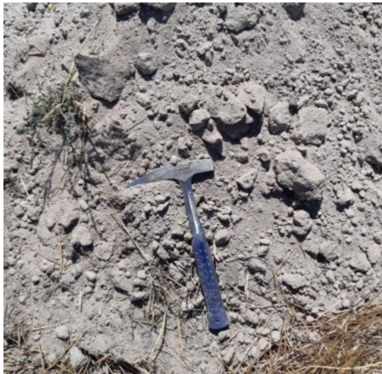
Figure 45: TP22 – Close-up of transported gravelly sand horizon.
