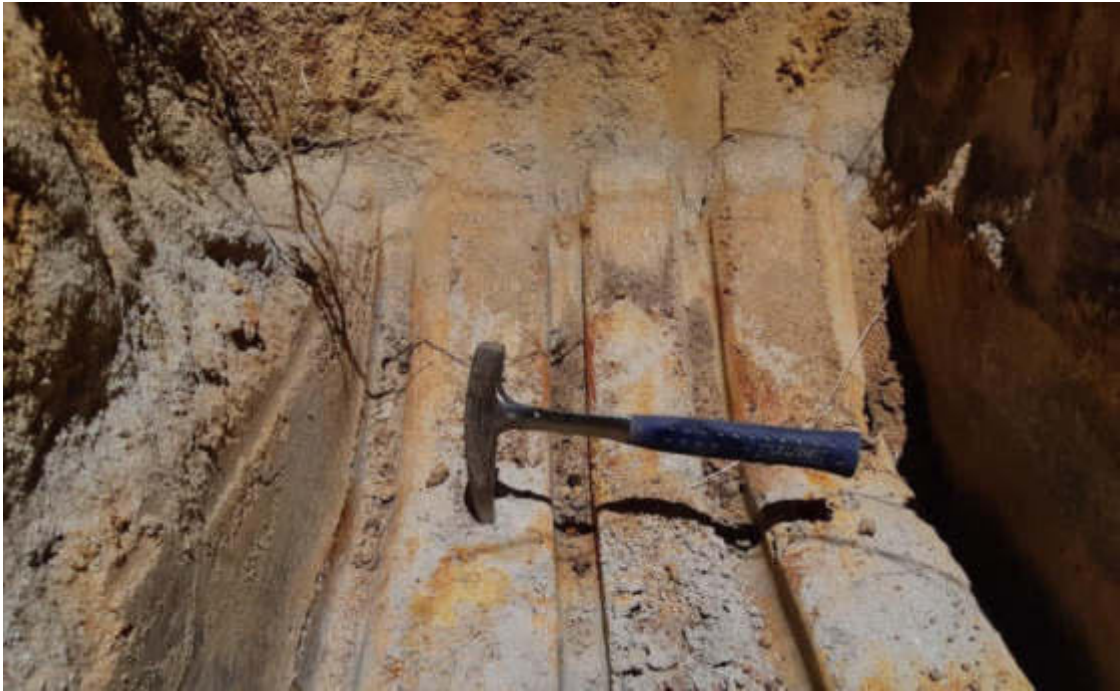
Figure 32: TP10 – Close up of bottom of trial pit; note sidewall smear near base of trial pit.
