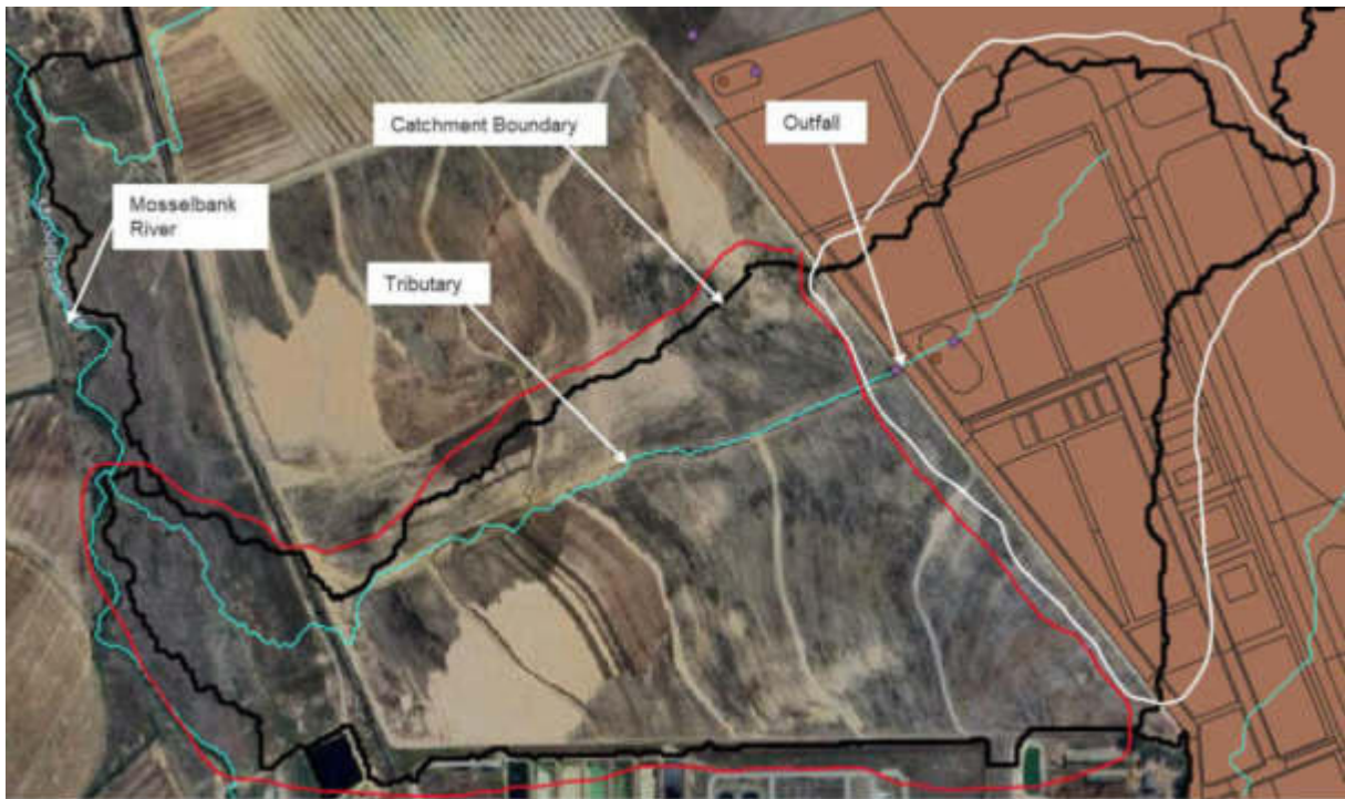
Figure 3-5: The portion of the catchment located inside the airport is bordered in white, and the rest of the catchment which will remain unchanged is bordered in red.
