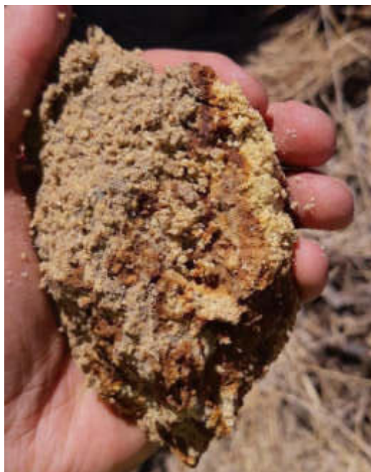
Figure 35: TP11 – Close-up of ferricrete nodule; note angular nature of grains stuck to nodule.
