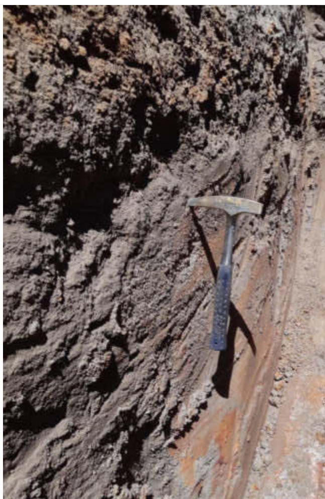
Figure 22: TP04: Close-up of trial pit sidewall. Note cemented nature of nodular ferricrete above hammer, and texture of sidewall ‘smear’ beneath hammer; sand- to clay- dominated with depth.
