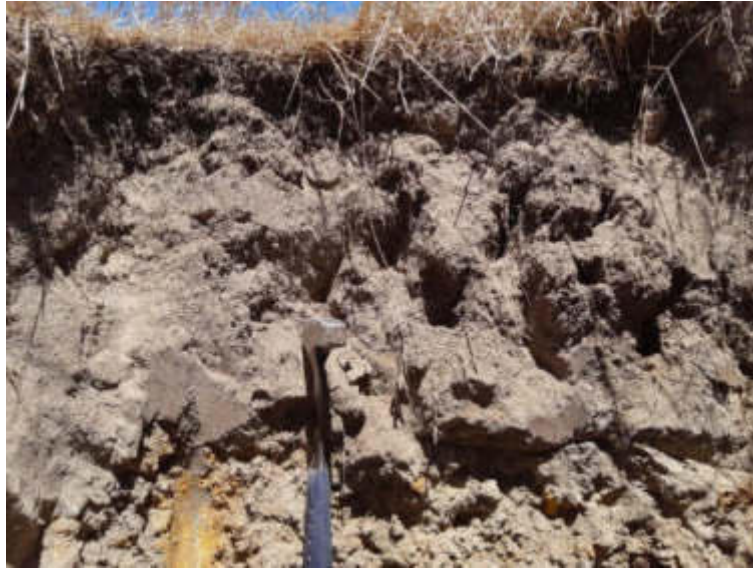
Figure 30: TP08 – Close-up of upper transported sand horizon.
