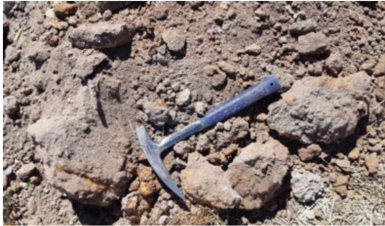
Figure 46: TP22 – Close-up of nodular ferricrete spoil pile; note this material excavated out in boulder-form occasionally. Excavation slow and time consuming.
