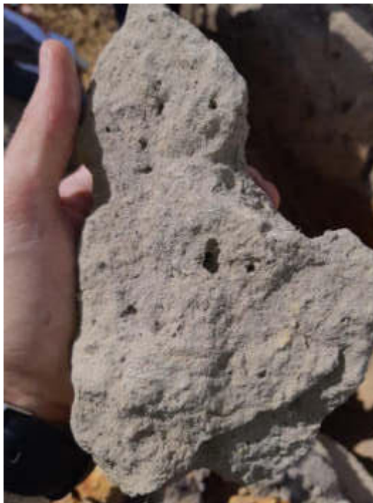
Figure 52: TP32 – Close-up of pin holed nature of transported material; likely due to bioturbation.
