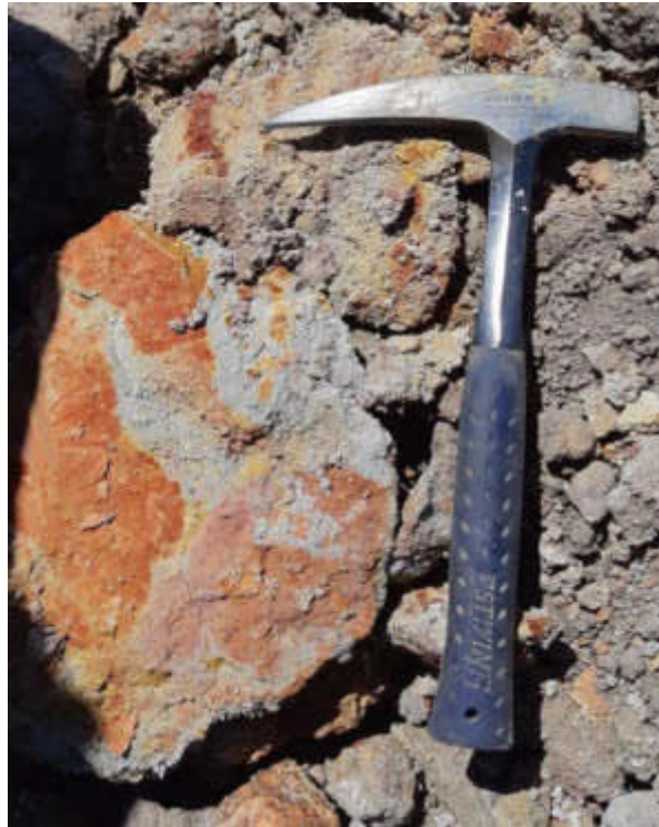
Figure 23: TP04 - Close-up of lower sandy clayey silt near base of trial pit.
