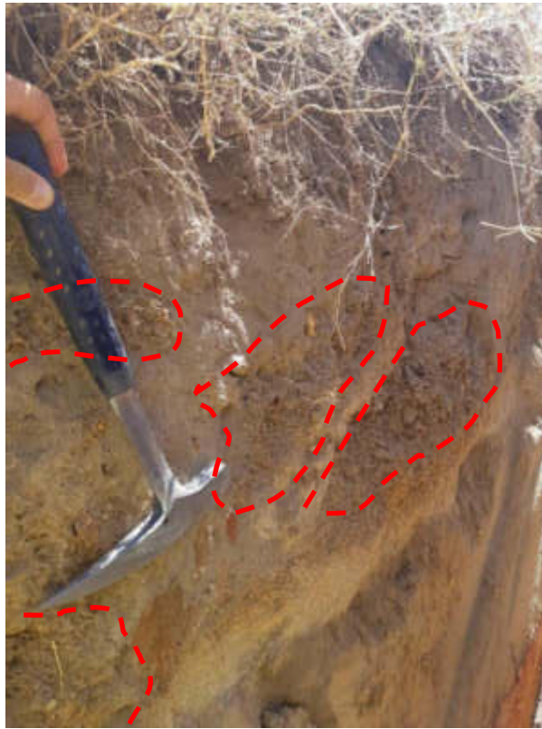
Figure 40: TP16 – Close-up of trial pit sidewall showing pockets of ferricrete nodules (annotated in red).
