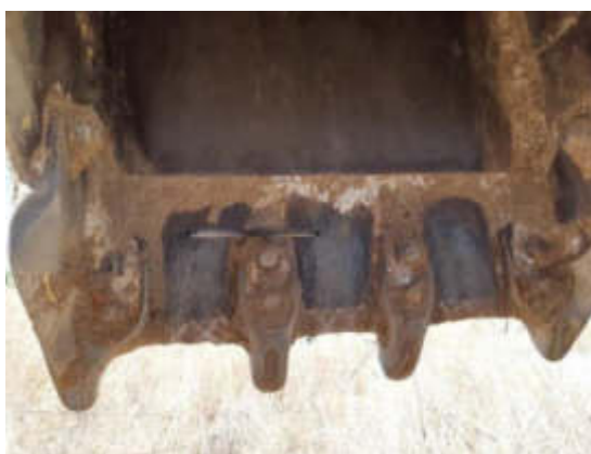
Figure 61: Close-up of TLB bucket tines used for conducting reconnaissance investigation.
