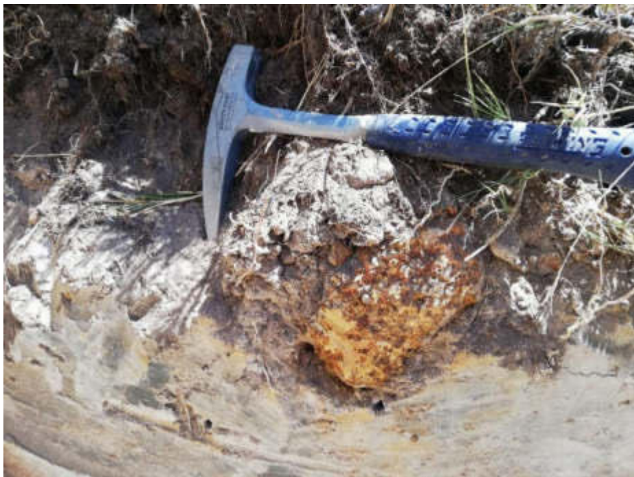
Figure 50: TP29 – Close-up of trial pit sidewall; note occasional indurated ferricrete boulders in upper-most horizon. Intense sidewall ‘smear’ in residual clayey sandy silt horizon.
