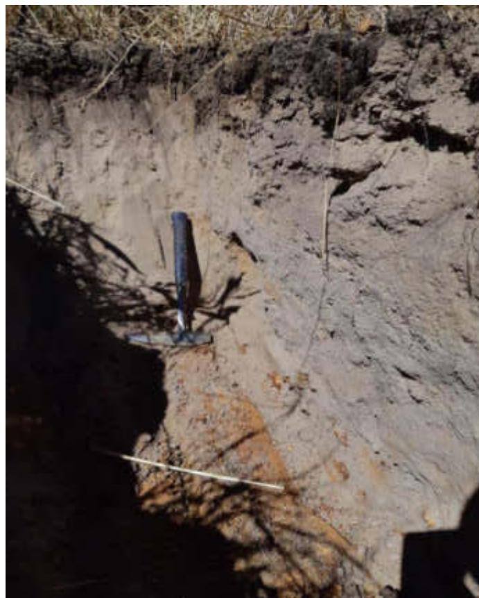
Figure 18: TP02 - Close-up of sidewall showing hardpan ferricrete refusal surface, note thin humified horizon on surface.
