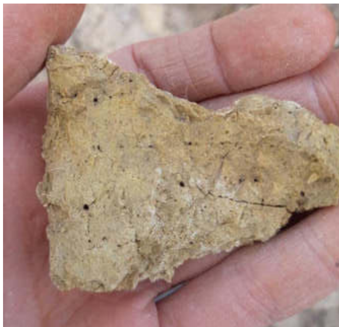
Figure 54: TP43 – Close-up of voided/bioturbated residual material.
