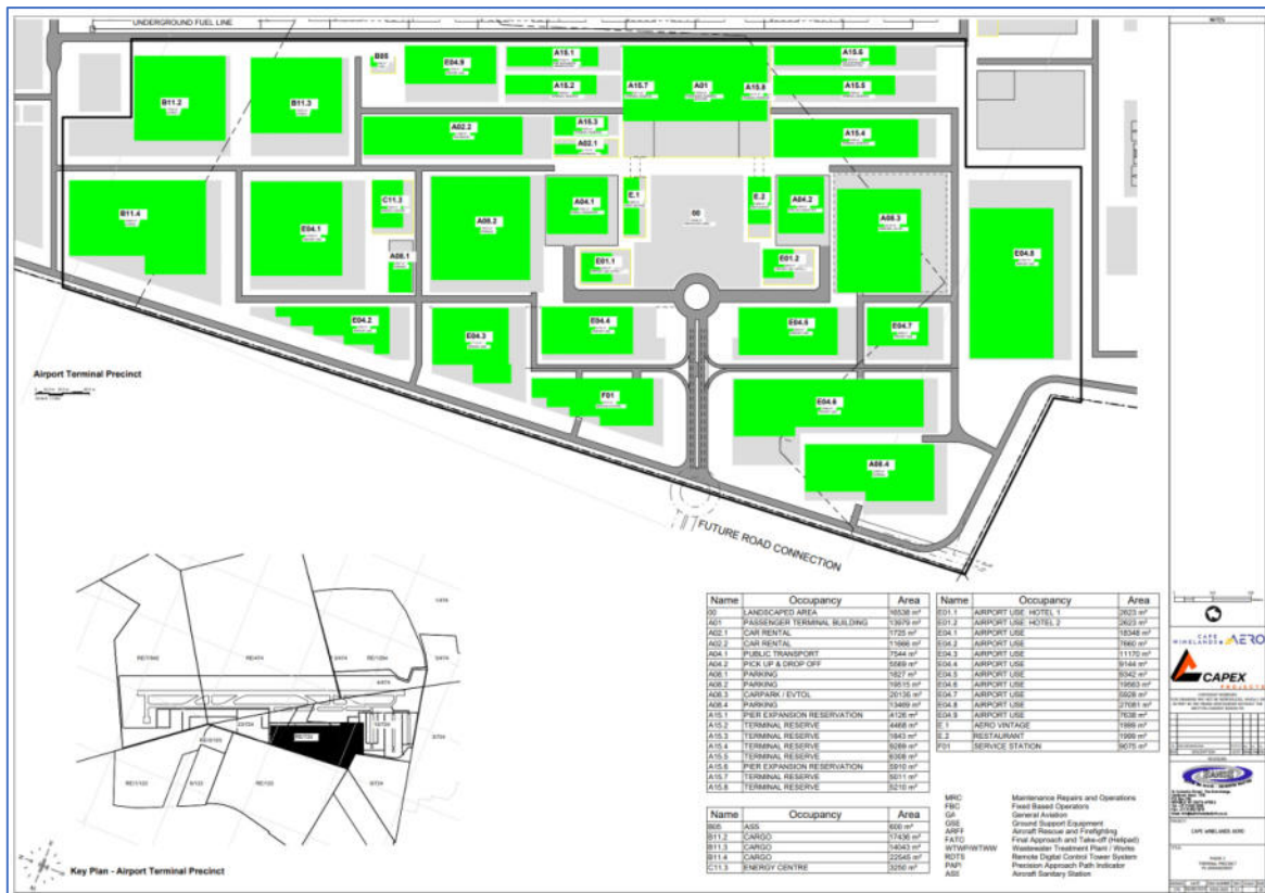
North End Airside PV Panel Locations
