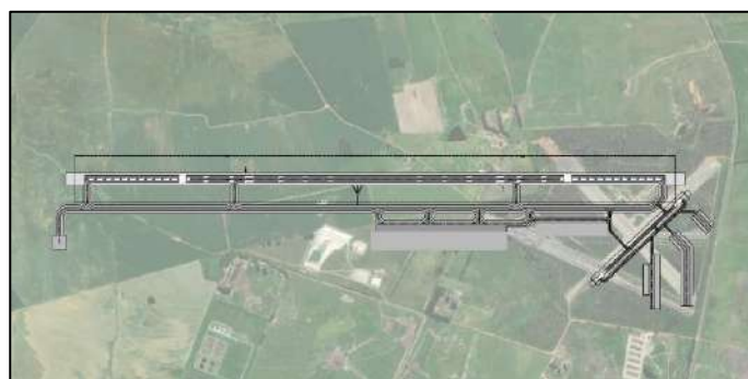
FIGURE 1: PLANNED RUNWAY LAYOUT IN PHASE 1 (CAPEWINELANDS AERO (PTY) LTD, 2023)
