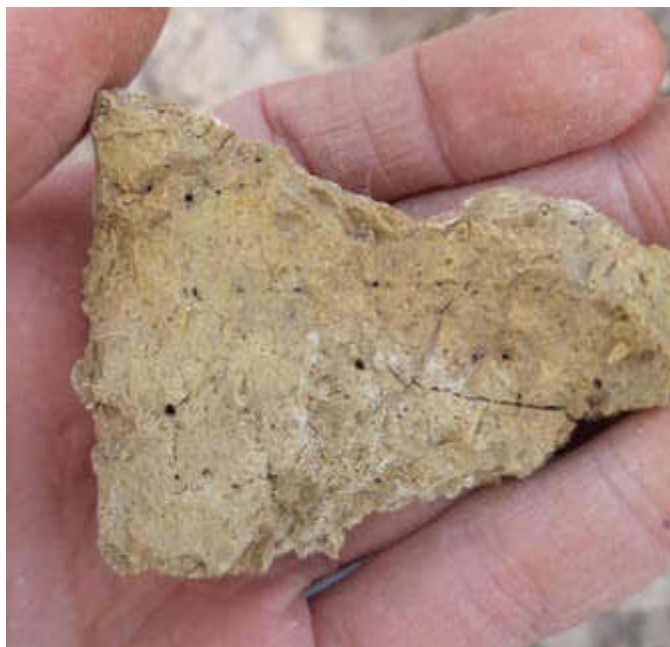
Figure 54: TP43 – Close-up of voided/bioturbated residual material.
