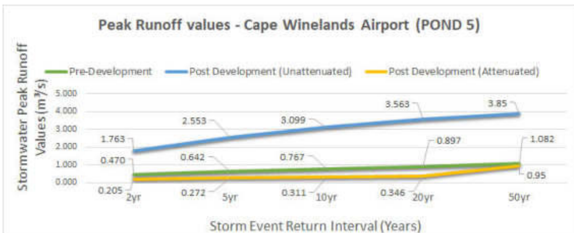
Figure 28: Pond 5 – Peak Run-off Values for Various Storm Events
