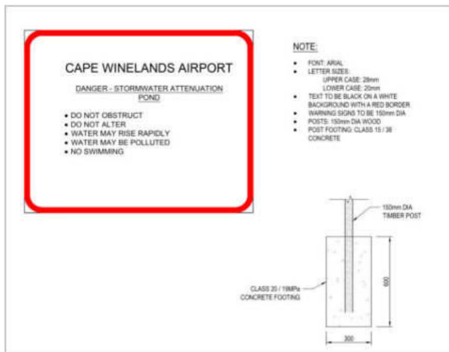
Figure 33: Typical Stormwater Pond Safety Signage
