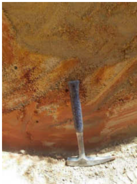
Figure 41: TP16 – Close-up of trial pit sidewall showing variation in 'smear' texture; material becomes less sandy toward base. Upon close inspection sandy grains are angular suggesting in-situ weathering.
