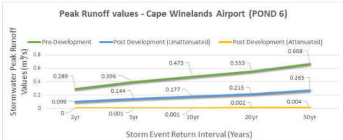
Figure 29: Pond 6 – Peak Run-off Values for Various Storm Events
