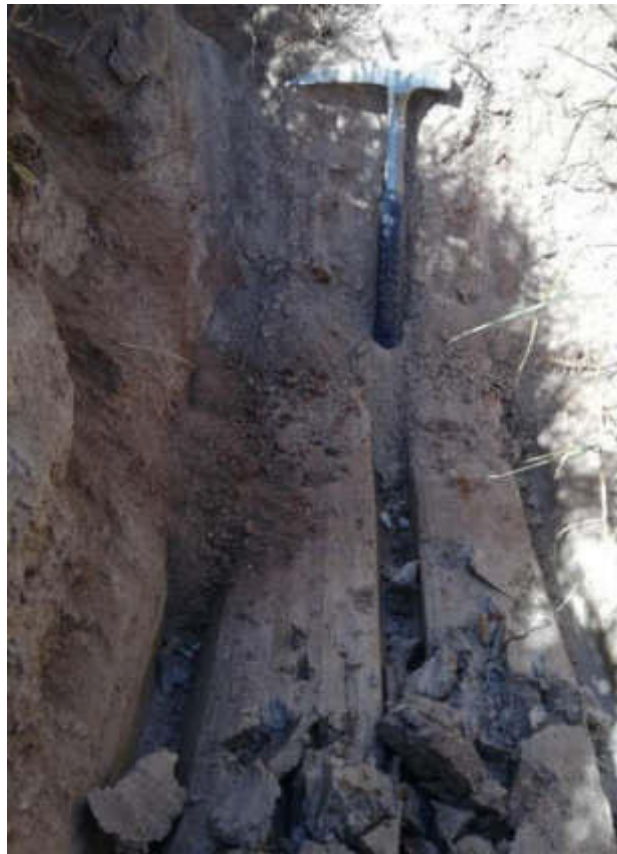
Figure 17: Close-up of TP01. Note cohesive nature of the material in the foreground, and the fine gravelly nature of material above refusal surface, i.e. next to hammer.
