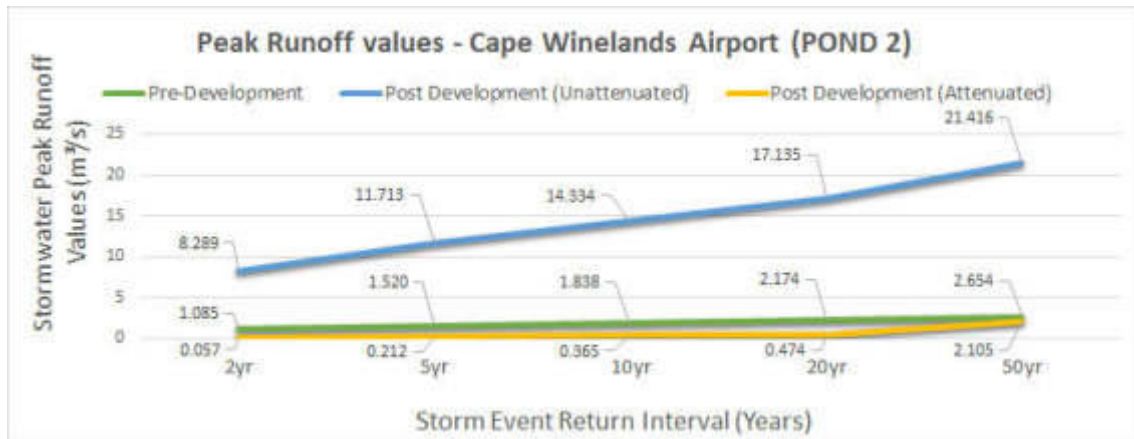
Figure 25: Pond 2 – Peak Run-off Values for Various Storm Events
