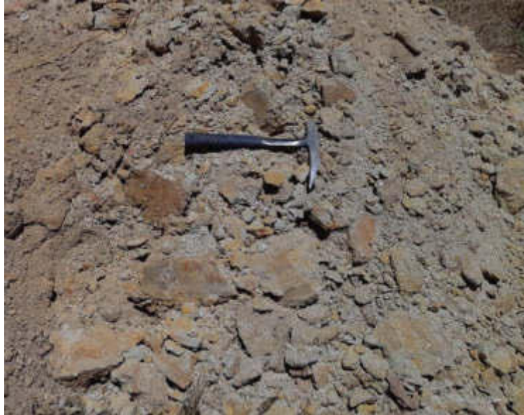
Figure 28: TP07 – Close-up of spoil excavated from residual horizon.
