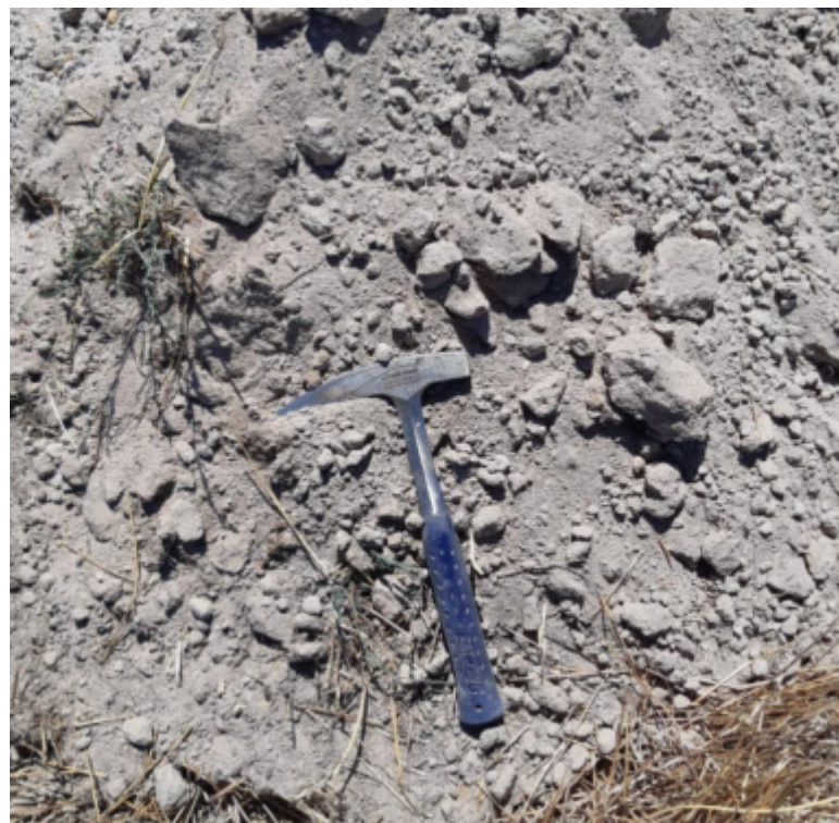
Figure 45: TP22 – Close-up of transported gravelly sand horizon.
