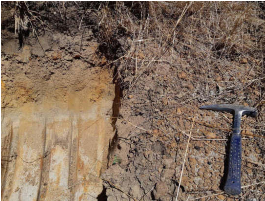
Figure 33: TP10 – Close up of bottom of ferricrete nodules strewn across surface surrounding trial pit; exposed soil profile pictured on LHS of photograph.
