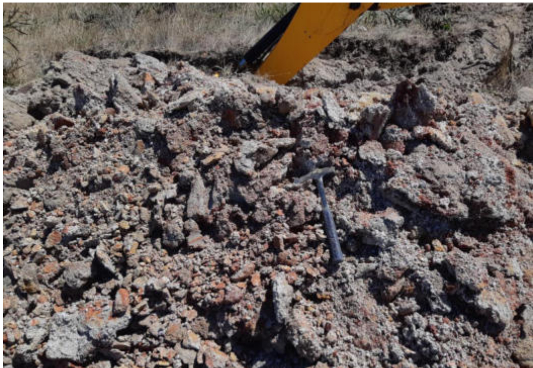
Figure 24: TP04 – Close-up of sandy clayey silt spoil.
