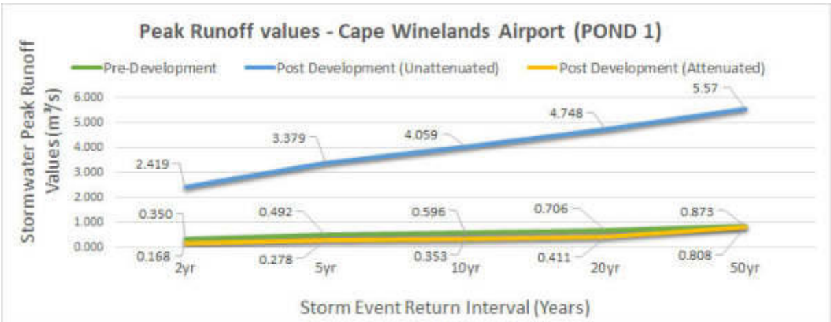
Figure 24: Pond 1 – Peak Run-off Values for Various Storm Events
