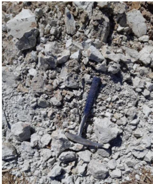
Figure 47: TP22 – Close-up of spoil of silty clay material of the residual horizon; note blocky form of material in foreground - evidence of relict foliations.
