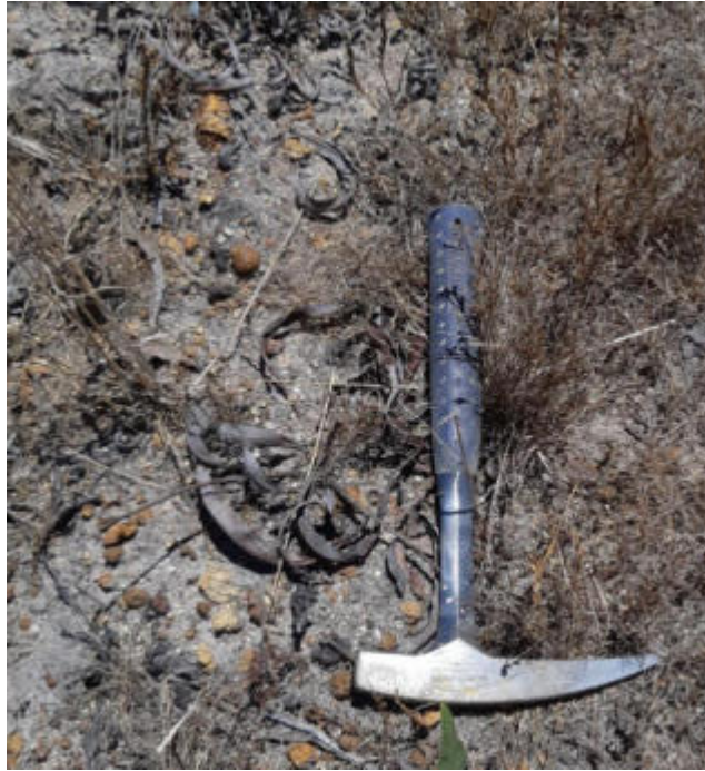
Figure 26: TP05 – ferricrete nodules scattered on surface.
