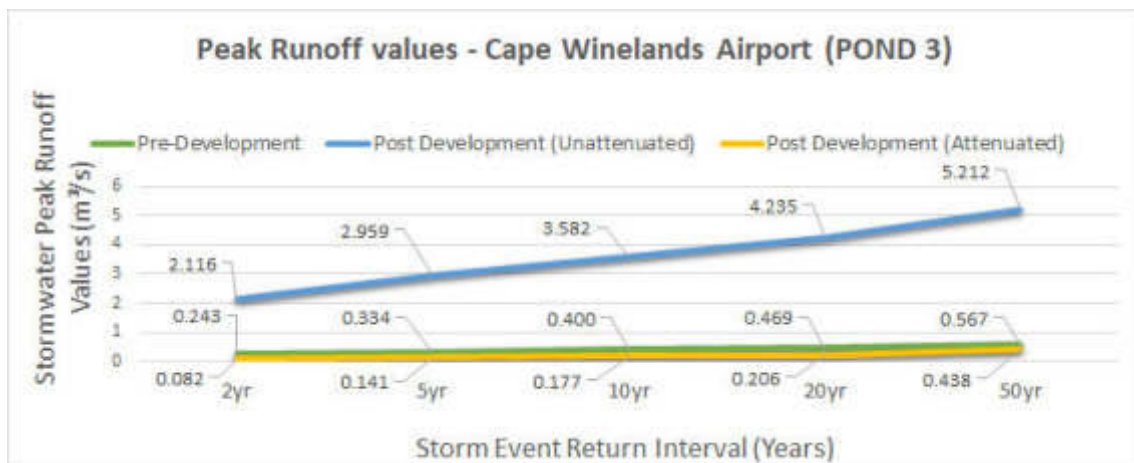
Figure 26: Pond 3 – Peak Run-off Values for Various Storm Events
