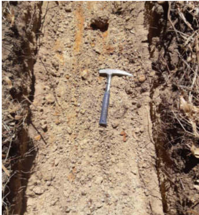
Figure 42: TP18 – Close-up of trial pit upper surface of red-orange-brown nodular ferricrete horizon prior to excavation through to silty clay residual horizon.
