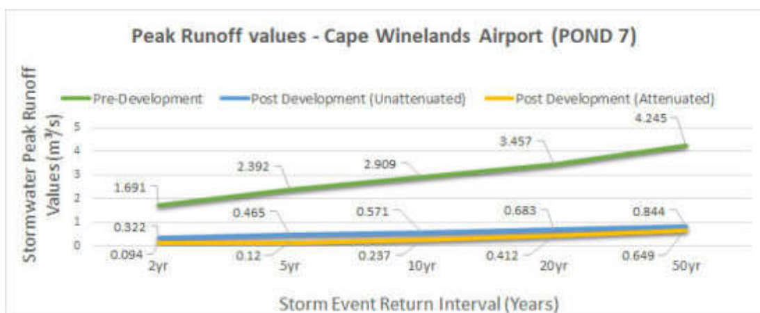
Figure 30: Pond 7 – Peak Run-off Values for Various Storm Events
