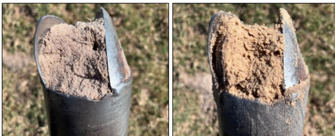
Figure 28: Saturation and low chroma identified within the (Left) first 30 cm of the soil; and (Right) > 30 cm of the soil samples taken from seep wetland.
