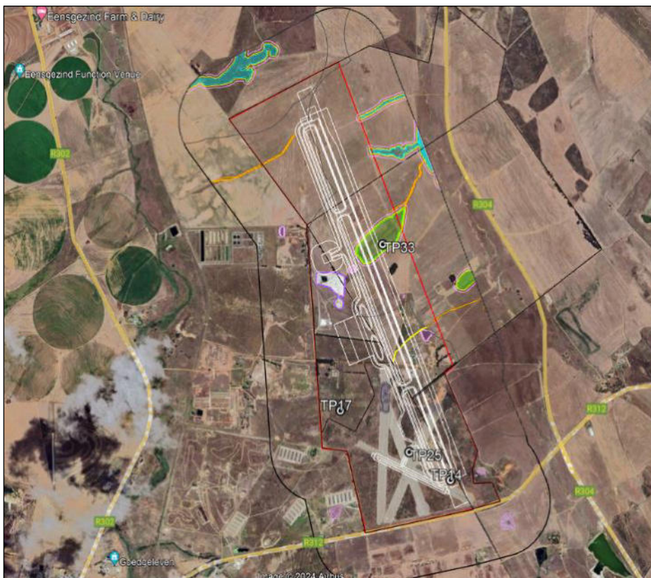
Figure 24: Test pits assessed by GEOSS (2023) for which a high water table was noted.
