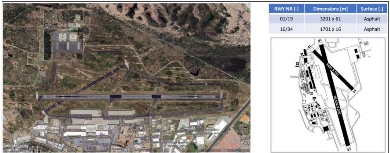
Figure 122: Aerial image of FACT and plan showing the two runways (NACO, ATNS, NLR, CONOPS report, Oct 2022)
