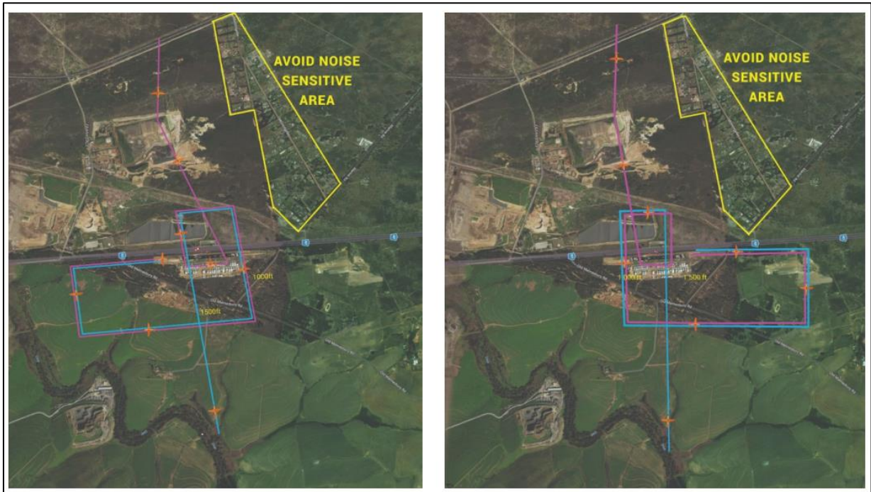
Figure 132: Charts indicating joining for Runway 02 (left) and 20 (right) - https://morningstarflyingclub.co.za/visiting-aircraft/ (NACO, ATNS, NLR, CONOPS report, Oct 2024)
