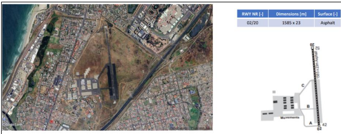
Figure 124: Aerial image of FAYP and plan showing the runway (NACO, ATNS, NLR, CONOPS report, Oct 2022)
