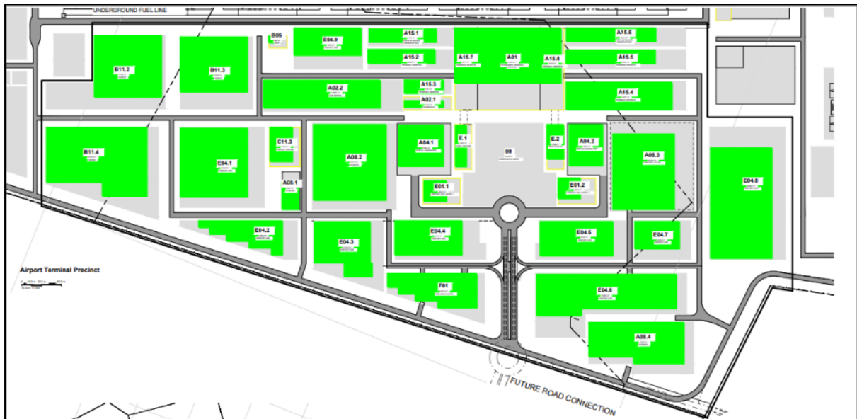
Figure 173: Proposed solar PV layout terminal precinct (SANDS, August 2024)
