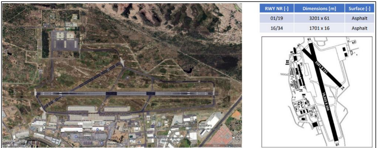
Figure 128: Aerial image of FACT and plan showing the two runways (NACO, ATNS, NLR, CONOPS report, Oct 2022)
