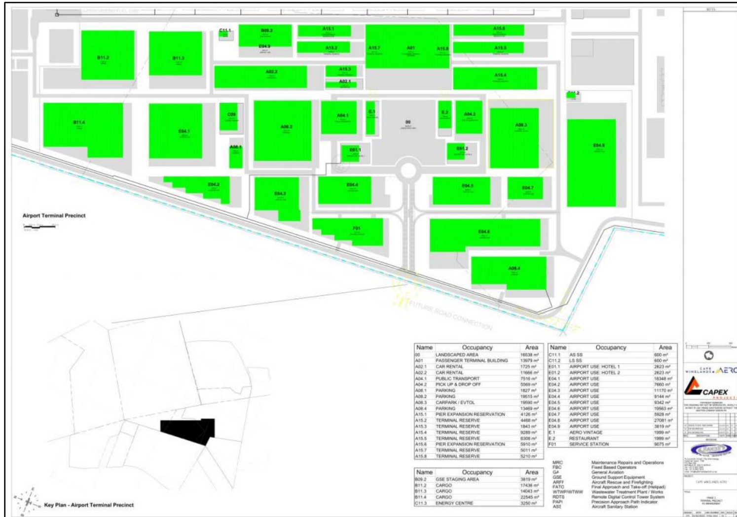
Figure 39: Terminal Precinct PV Plant (PV arrays in GREEN shading) (SANDS, Electrical Bulk Services, February 2025)
