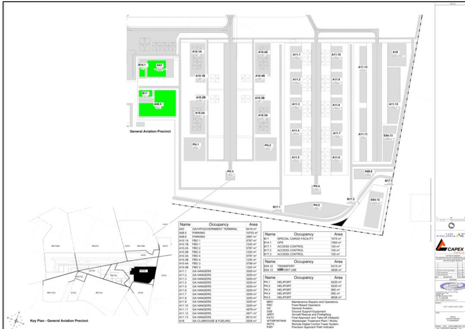
Figure 41: General Aviation Precinct PV Plant (PV arrays in GREEN shading) (SANDS, Electrical Bulk Services, February 2025)
