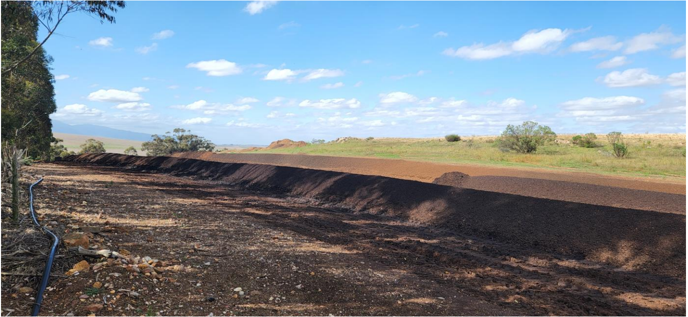
Figure 5: Composting wind rows that a regularly mixed and watered (when required) to improve oxygen content, to mix in or remove moisture and to redistribute cooler and hotter portions of the pile.
