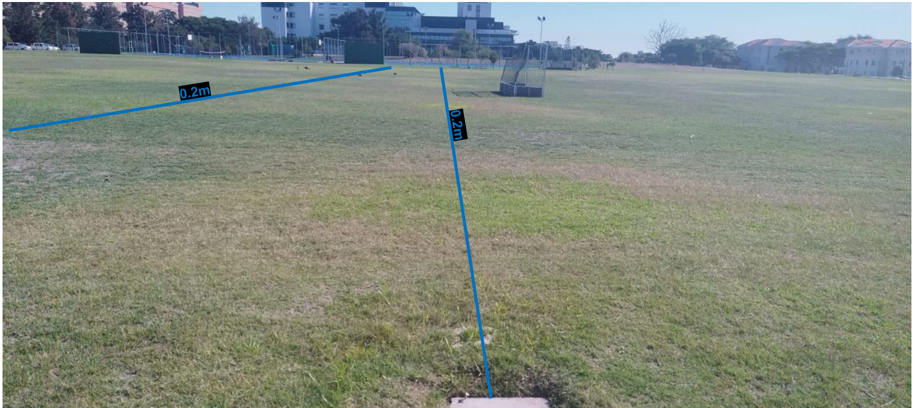
PHOTOGRAPH 5: Area Scanned Showing Utilities Found and Depths – View Looking West
