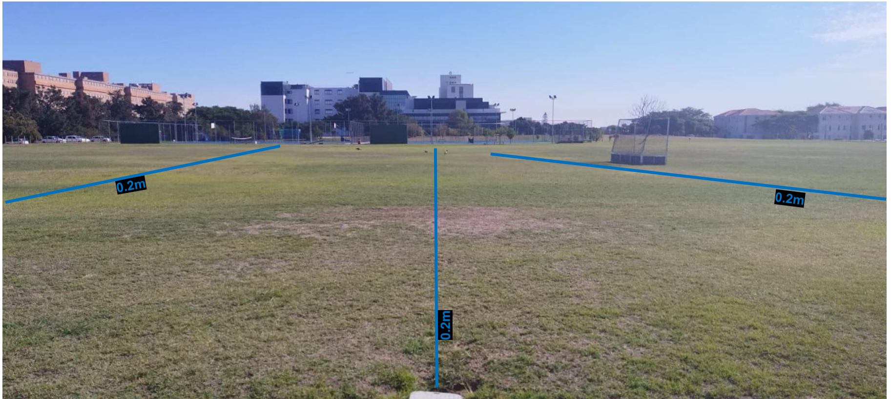
PHOTOGRAPH 6: Area Scanned Showing Utilities Found and Depths – View Looking West
