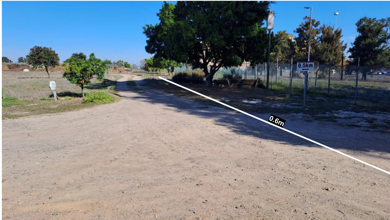
PHOTOGRAPH 16: Area Scanned Showing Utilities Found and Depths – View Looking South
