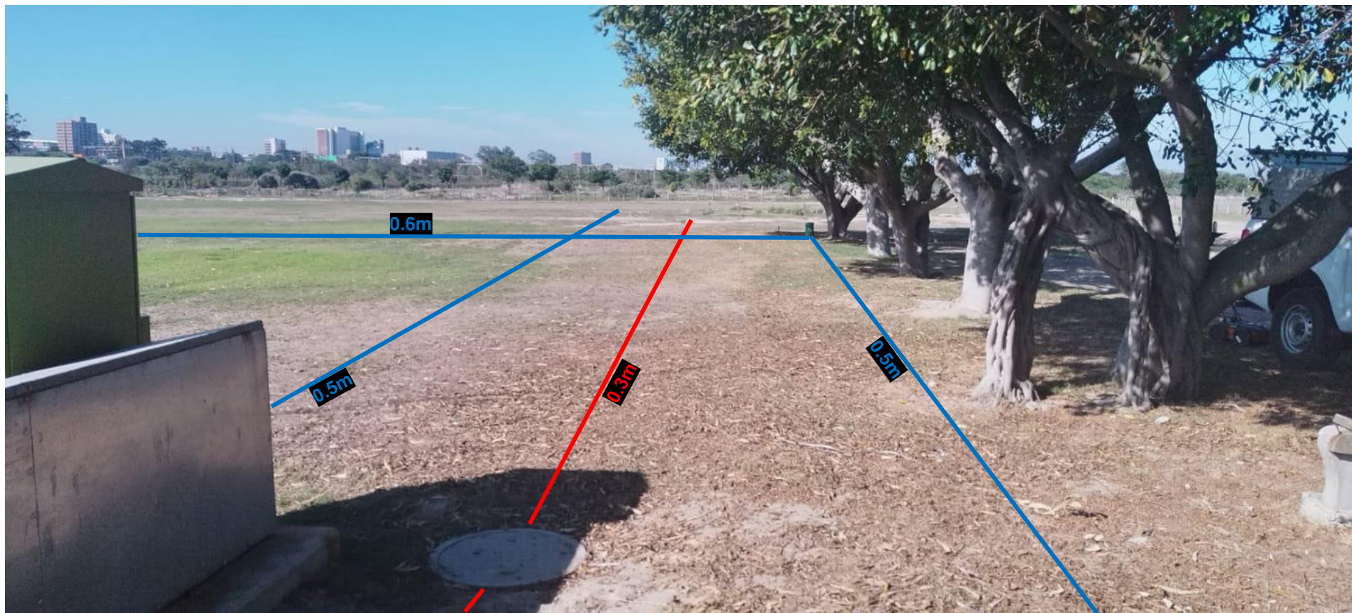
PHOTOGRAPH 2: Area Scanned Showing Utilities Found and Depths – View Looking East
