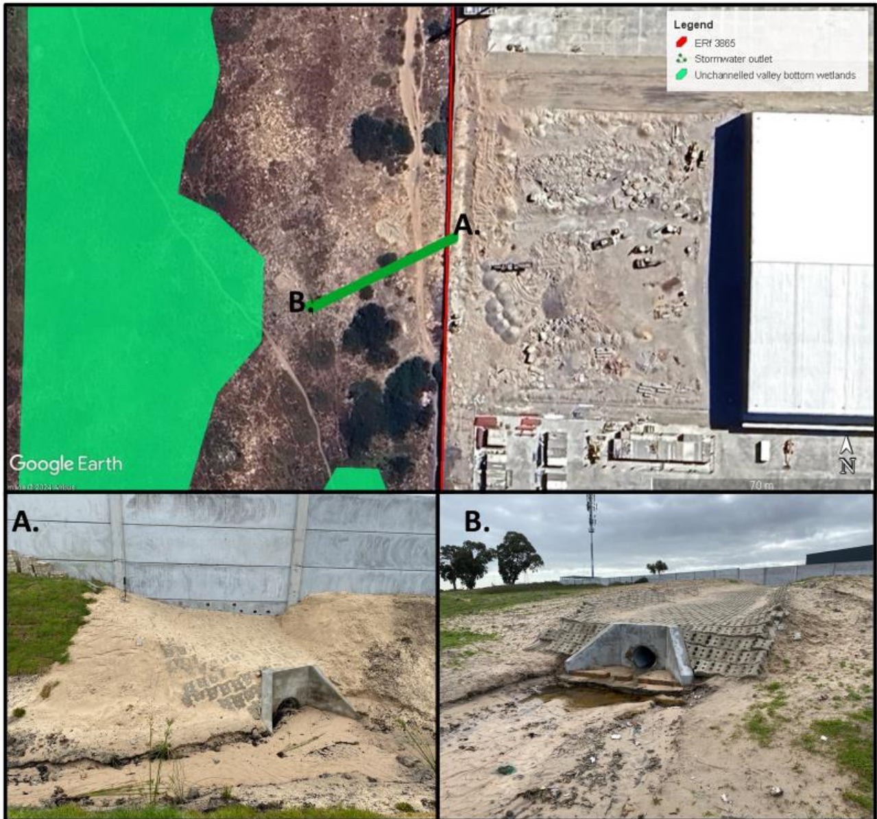
Figure 14. A Google Earth satellite image of the western boundary of the site showing the location of the stormwater outlet from the attenuation pond, A) the inlet to the stormwater outlet pipe within the attenuation pond and B) the outlet from of the stormwater outlet into the Kuils River corridor, showing erosion downstream of the outlet.
