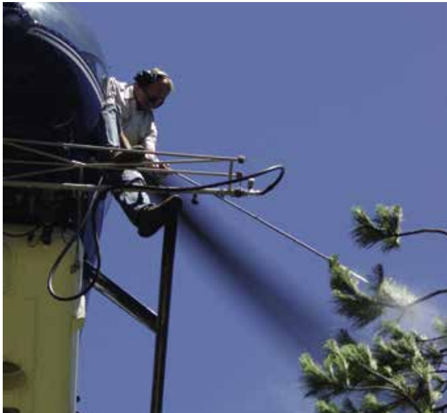
Applying herbicide from a helicopter using the wand method is the most targeted, although it is still under development. © Andrew Turner
