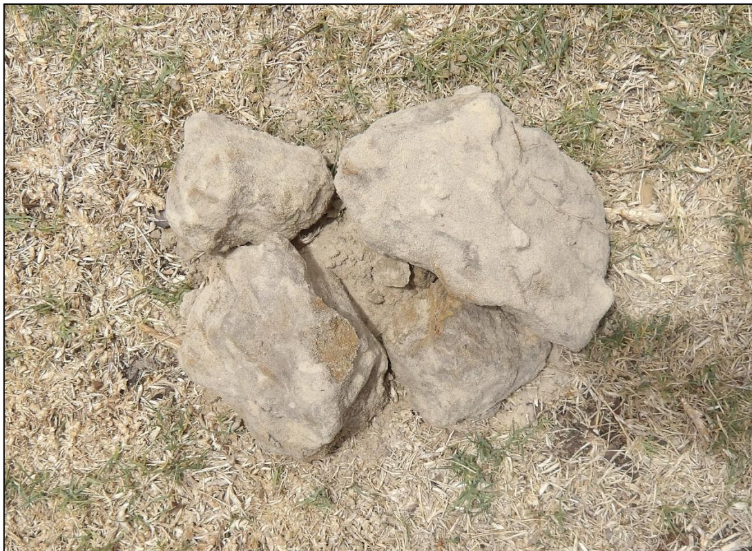
Figure 15: Clay lumps removed from the T3 excavation at 1.6 m depth.
