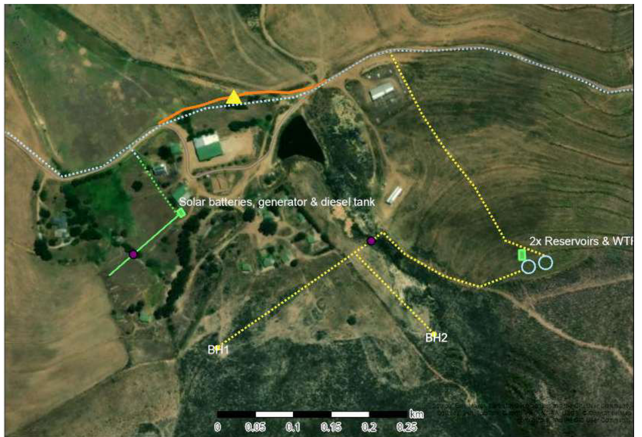
Figure 14: Showing the new revised layout within the Farmyard (the yellow triangle depicts the proposed suspended bridge location and the two purple dots indicate the stream crossings).
