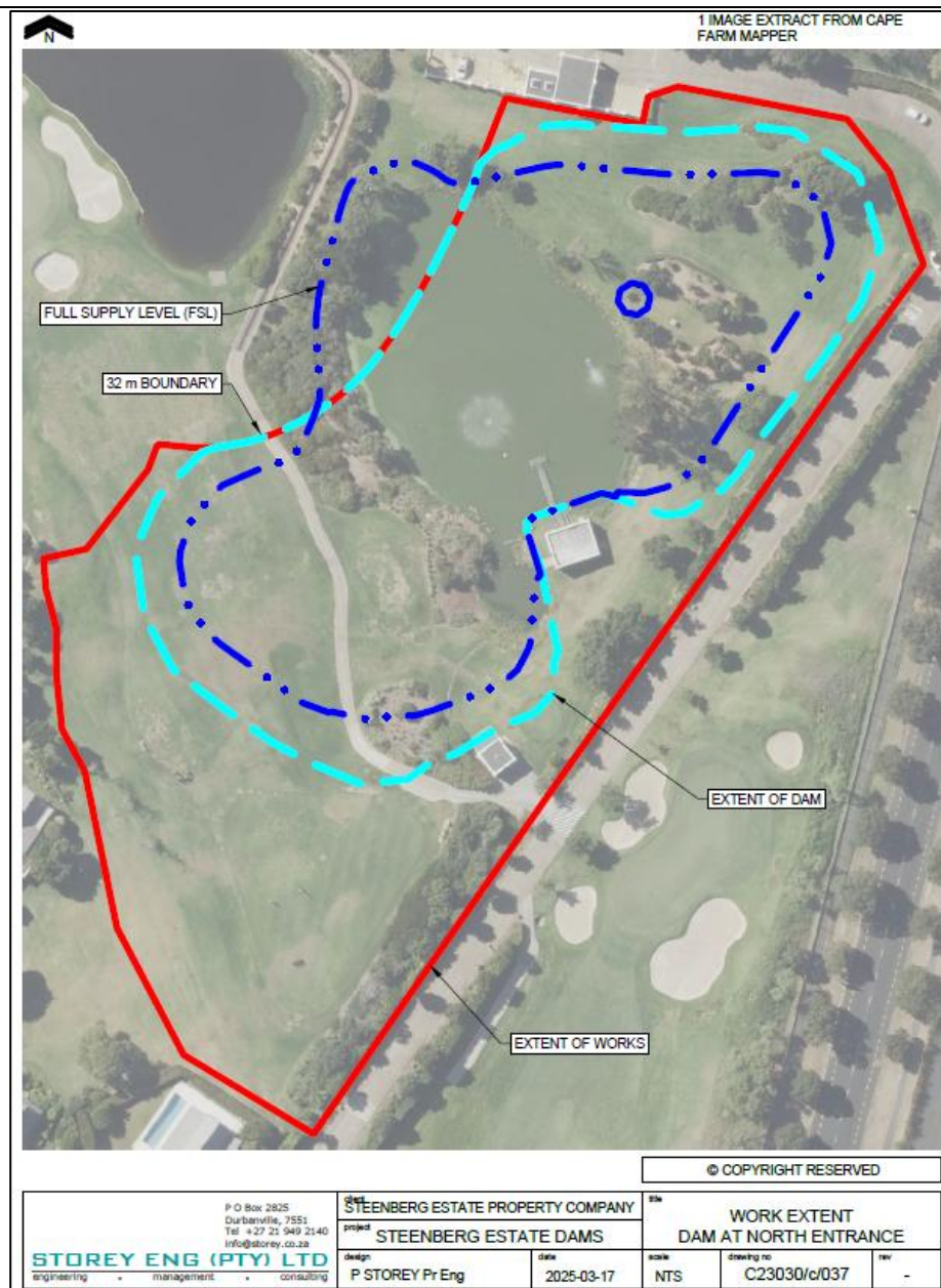
Figure 6: Extent of the work area, dam perimeter and full supply level of the Northern Entrance Dam
