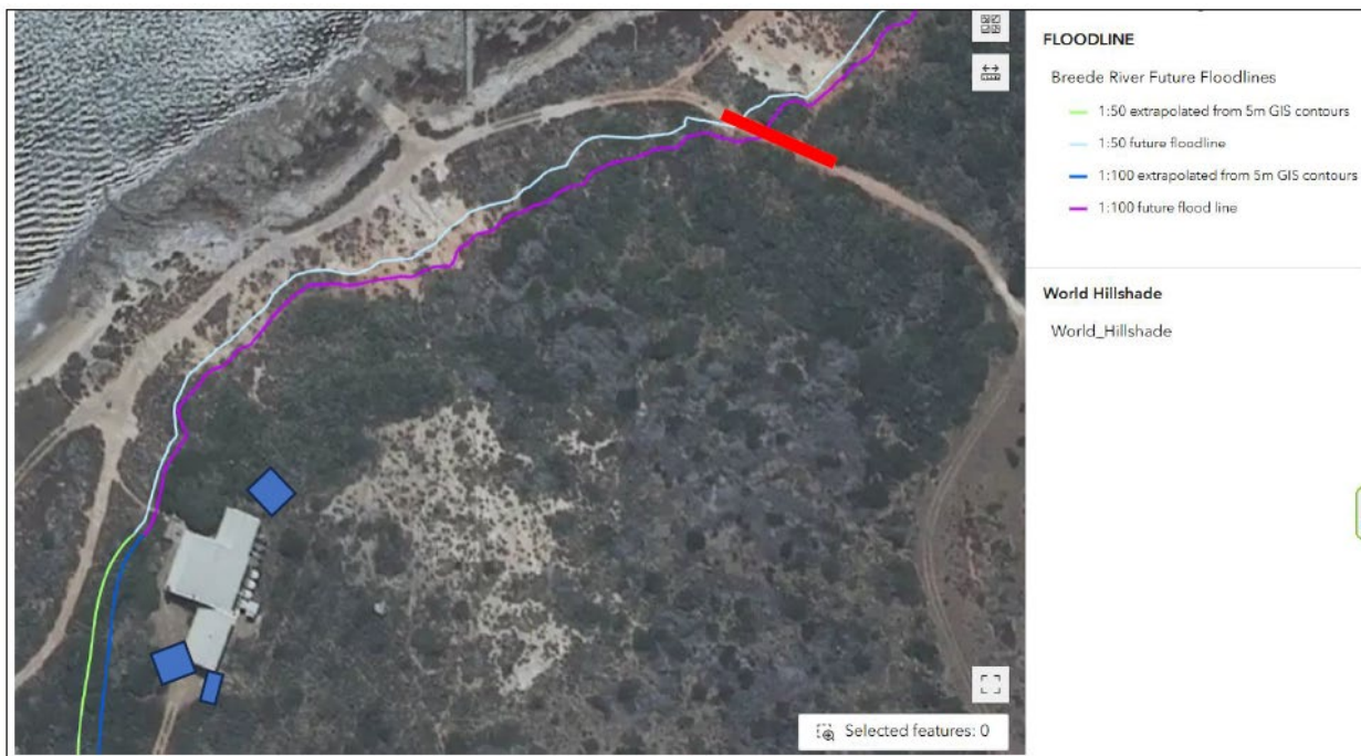
Figure 4c: Farmhouse and new footprints in blue is above the flood lines, the road in red is existing and works will be like for like.
