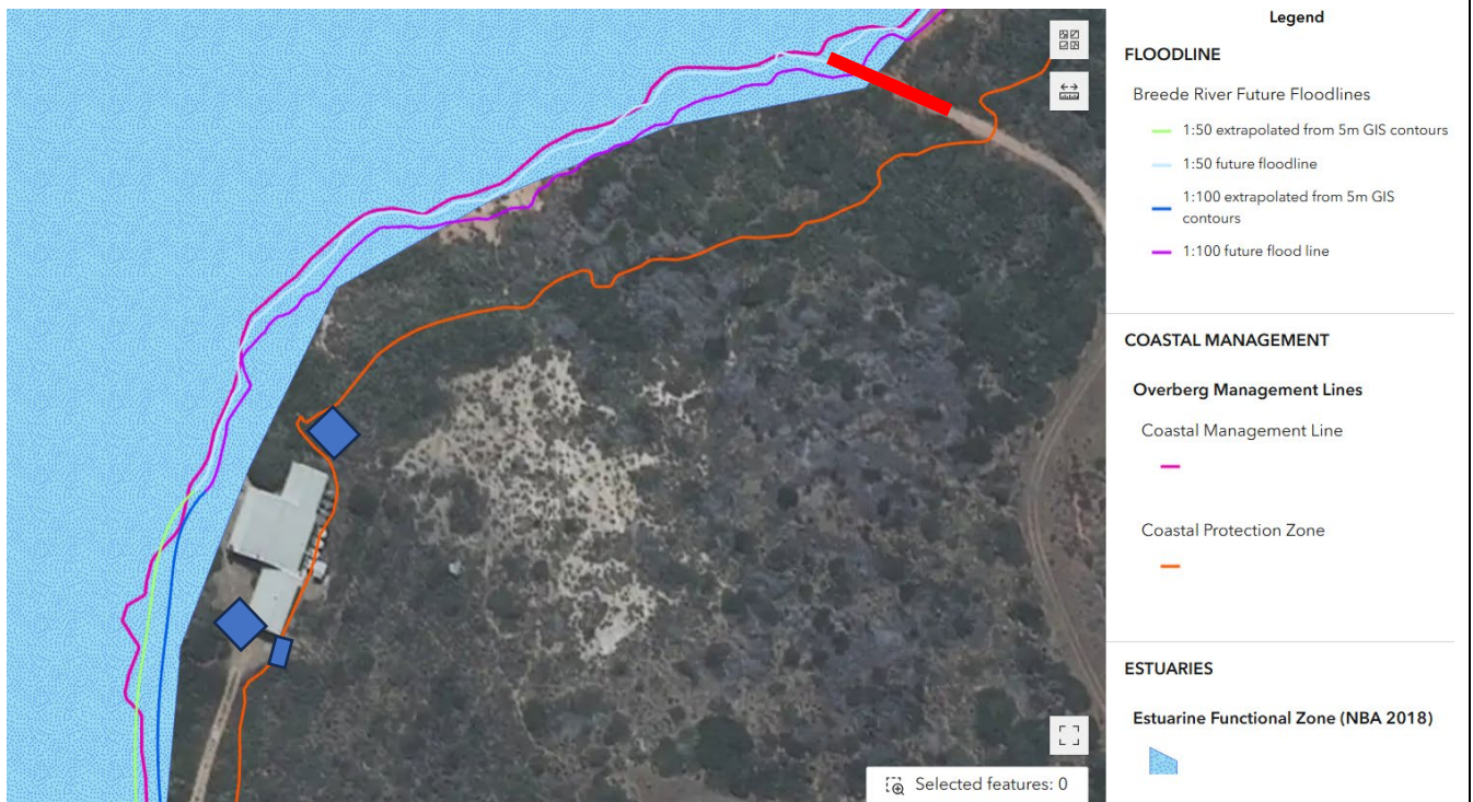
Figure 13: Map showing that all the lines discussed under Figure 10, 11 & 12 in relation to the approx. position of the proposed areas of work; blue new units and parking and red road section requiring resurface.
