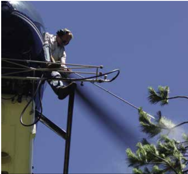
Applying herbicide from a helicopter using the wand method is the most targeted, although it is still under development. © Andrew Turner
