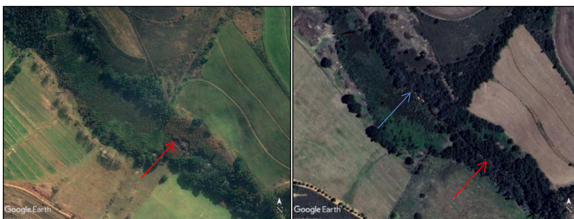
Figure 8: Google Earth images indicating the start of the headcut erosion in 2009 (left – red arrow) and the start of the headcut erosion in 2024 (right – blue arrow, with red arrow indicating initial 2009 start).
