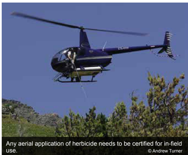
Applying herbicide from a helicopter using the wand method is the most targeted, although it is still under development. © Andrew Turner
