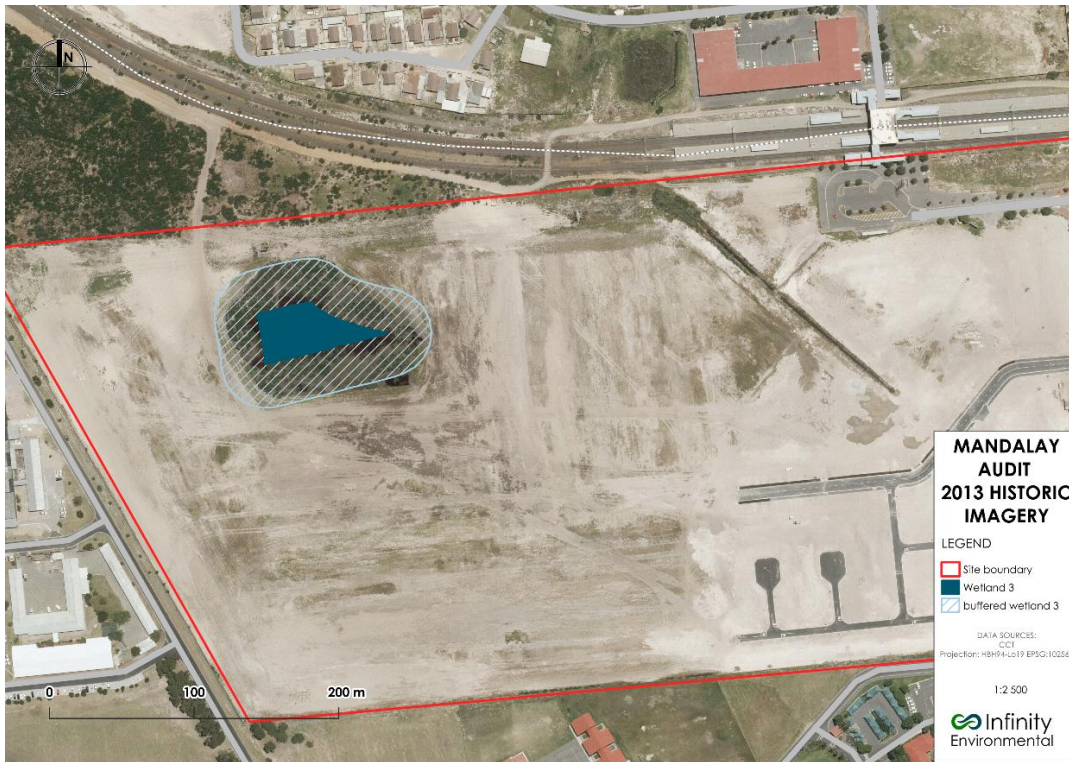
Figure 1: Wetland 3 delineated in the Freshwater Specialist Report. The figure shows the wetland and the buffer during the initial site clearance in 2013
