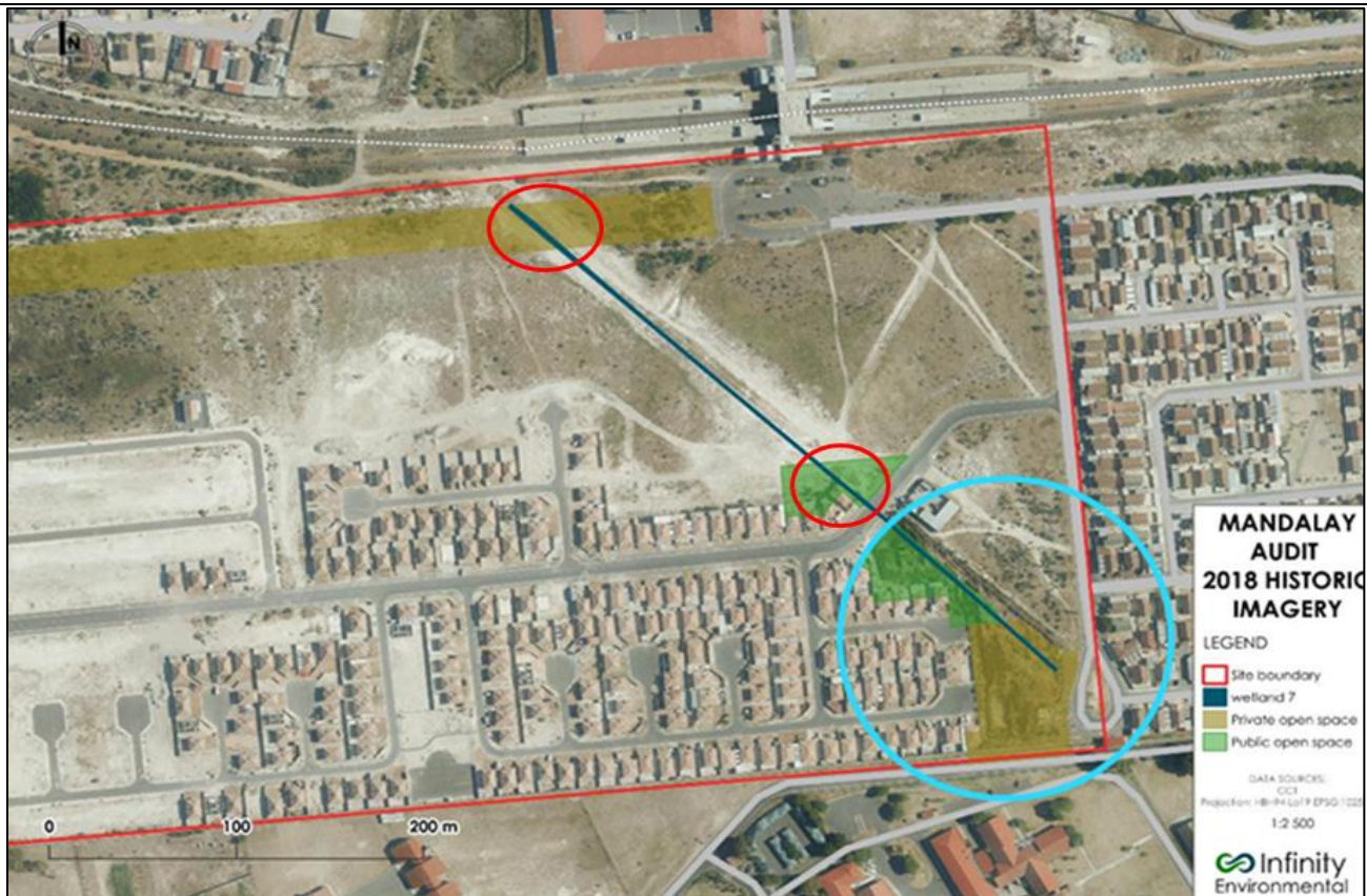
Figure 4: In 2018, the Wetland 7 was piped up to the offset area shown in the blue circled area (Infinity Environmental, 2025). The portions of wetland 7 encircled in red were not approved for piping in terms of NEMA.
